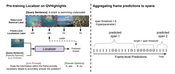
Figure 6: Left: For LOCALIZER pre-training, we utilize the video moment retrieval labels for the keyframe localization task. **Right:** we aggregate LOCALIZER's frame-level predictions into video-level span predictions.
