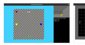
Figure 3: Visualization of the miniworld-gotoobj-env (left) and minigrid-gotoobj-env (right). The miniworld-gotoobj-env image shows both the top-down view and the agent view (top-right window). During training the agent only has access to the agent view of the environment.
