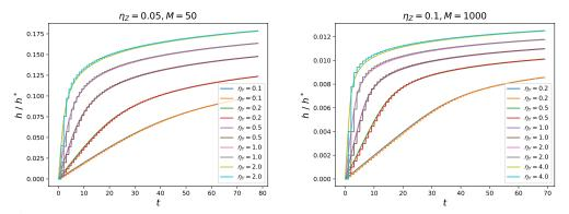
Figure 8: Numerical simulation of  $h^*$  and h with changing  $\eta_Y$ . The stepped folded line represents  $h^*$  and the smooth curve represents h. The gap between  $h^*$  and h is bounded and goes to zero when time grows.
