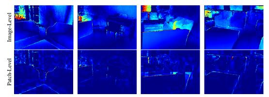
Figure 1: Error map visualization of image-level and patch-wise scale and shift adjustment: relative depth map in various viewpoints is fitted in two ways, image-level fitting (first row) and patch-level fitting (second row).
