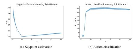
Figure 4: An illustration of the plateau effect with stacking more frames (s). We show this effect on two tasks, keypoint estimation (measured in MLE loss) and action classification (measured in Top1 accuracy). We generally pick the turning point as the optimal stacking, as this offers a good balance between performance and run-time efficiency. The detail is discussed in Section 4.2.
