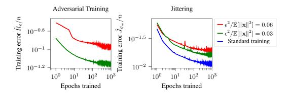
Figure 13: Training metrics of U-nets for adversarial training, jittering and standard training. The plot shows that the convergence rates are very similar for the considered setup. The curves show the training of networks for perturbation levels  $\epsilon^2/\mathbb{E}[\|\mathbf{x}\|^2] = 0.03$  (red) and 0.06 (green). Training the methods takes roughly 600 epochs for convergence.
