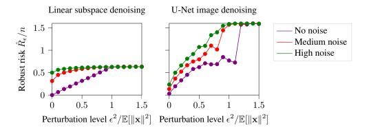
Figure 7: The empirical robust risk for models trained with adversarial training for noise levels  $\sigma_z=0$  (no noise),  $\sigma_z/\sqrt{n}=0.5$  (medium noise) and  $\sigma_z/\sqrt{n}=1.5$  (high noise). The transition predicted by Theorem 3.1 at  $\epsilon^2\approx\mathbb{E}\left[\|\mathbf{x}\|_2^2\right]$  for the estimator to map to zero occurs for the subspace and image denoising settings.
