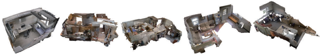
Figure 8: Mesh visualization. MVDiffusion first generates RGB images given depths/poses and then fuse them into mesh with TSDF fusion.
