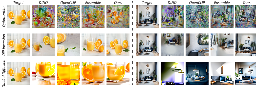
Figure 10: Feature inversion across different metrics and image priors. Given a target image, we optimize for an image, where the objective is to match the target image embedding of a given backbone. Without any image prior (Optimization), our metric better recovers the color, shape and semantics of the target image. With a weak image prior [83, 84] (DIP Inversion), our metric is able to reproduce scene structure and semantics. Using a diffusion model [22] as a strong prior, our metric better captures overall semantics and scene appearance.
