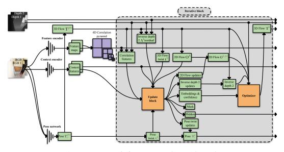
Figure 4: Drunkard's Odometry architecture in detail.
