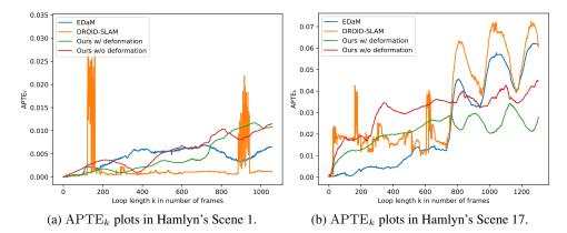
Figure 6: Camera tracking performance on the Hamlyn dataset. APTE<sub>k</sub> values along the N different k-frames-length-loops in Hamlyn's scenes 1 (a) and 17 (b) for EDaM [9], DROID-SLAM [34] and Drunkard's Odometry (ours) with and without having been trained in deformable scenes of the Drunkard's Dataset (i.e. trained in level 1 and 0, respectively). The training on deforming scene substantially improves the performance of our method.
