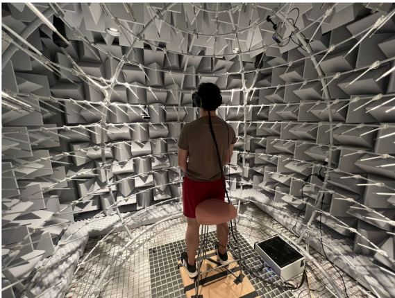
Figure 2: Capture stage with five body-tracking cameras and 345 microphones on a sphere around the participant.
