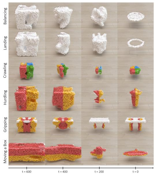
Figure 11: Demonstrations of generations changing from noises to robots with physical utility throughout the diffusion sampling process. We present snapshots at diffusion times t = 600, 400, 200, 0 for all presented tasks.
