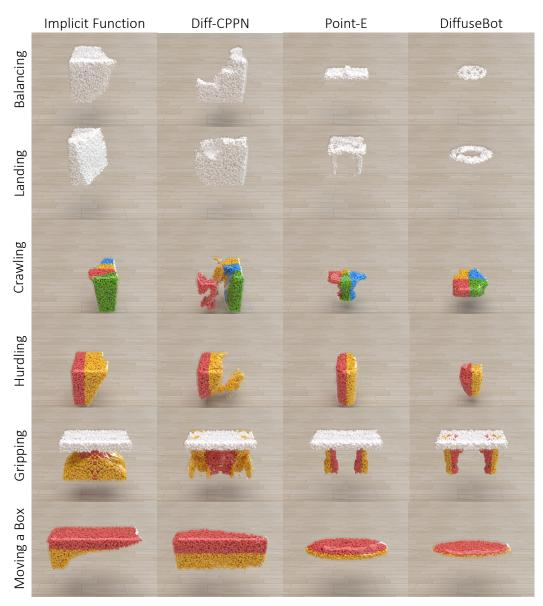
Figure 12: Comparison of robots generated by different baselines.
