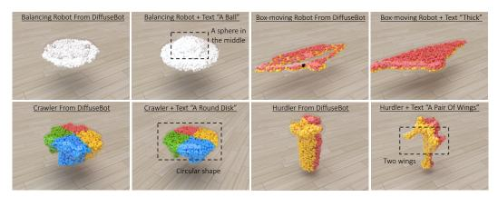
Figure 13: More examples of incorporating human textual feedback into robot generation by DiffuseBot.
