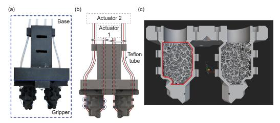
Figure 14: (a) shows a fabricated proof-of-concept physical robot gripper; (b) describes detailed robot configuration; (c) represents interior structure design used to soften the robot body.
