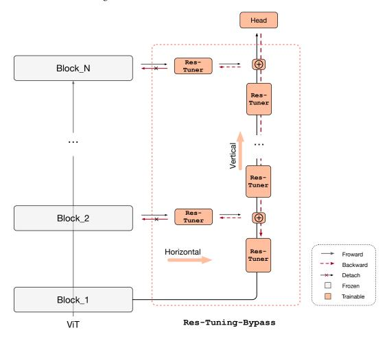
Figure 8: Architecture design for discriminative tasks.
