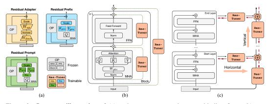
Figure 3: **Structure illustration** of (a) various Res-Tuners in our unbinding form, (b) our Res-Tuning framework that is flexible and efficient, and (c) Res-Tuning-Bypass, the memory-efficient version of our framework.
