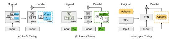
Figure 2: **The original and the unbinding form** of (a) prefix tuning [41], (b) prompt tuning [28], and (c) adapter tuning [25] for parameter-efficient transfer learning.
