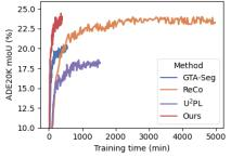
Figure 3: **mIoU** (%) vs. training time. Ours shows clear efficiency over the competing methods with a much improved final mIoU.
