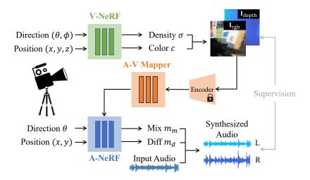
Figure 2: The pipeline of our method. Given the position (x, y, z) and viewing direction  $(\theta, \phi)$  of a listener, our method can render an image the listener would see and the corresponding binaural audio the listener would hear. Our model consists of V-NeRF, A-NeRF, and AV-Mapper. A-NeRF learns to generate acoustic masks, V-NeRF learns to generate visual frames, and AV-Mapper is optimized to integrate geometry and material information extracted from V-NeRF into A-NeRF.
