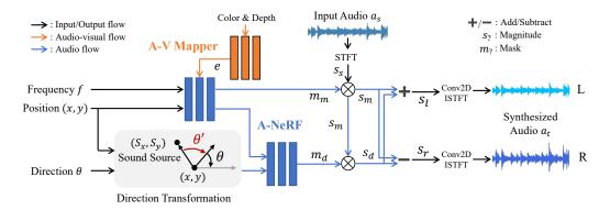
Figure 4: The pipeline of A-NeRF. Given the 2D position (x, y) and direction  $\theta$  of a camera pose, A-NeRF can render mixture mask  $\mathbf{m}_m$ , and difference mask  $\mathbf{m}_d$ , which then be used for audio synthesis. A-NeRF is also composed of two MLPs, with the first predicting mixture mask  $\mathbf{m}_m$  and the second estimating difference mask  $\mathbf{m}_d$ . The direction  $\theta$  is transformed relatively to the sound source prior to inputting into A-NeRF.
