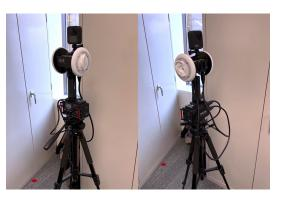
Figure 9: Recording system. It comprises a professional binaural microphone, a sports camera, and a recorder.
