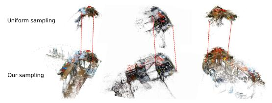
Figure 3: **3D reconstructions with different sampling.** We compare three scenes reconstructed using either uniform frame selection or our homography-based pipeline. Uniform sampling yields partial reconstructions with limited coverage. Ours demonstrates superior performance, resulting in better coverage by registering successfully more viewpoints.
