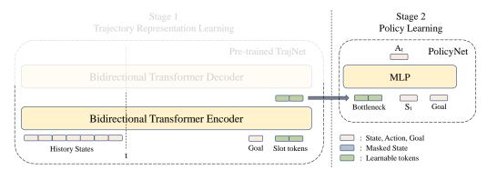
Figure 2: **Stage 2 – Policy Learning.** We implement policy learning with a simple MLP as PolicyNet. We input unmasked history states and retrieve the bottleneck from pre-trained encoder. Then the bottleneck is taken as the input to the policy network. We view the bottleneck generated by pre-trained encoder as goal-conditioned latent representations for the future trajectory.
