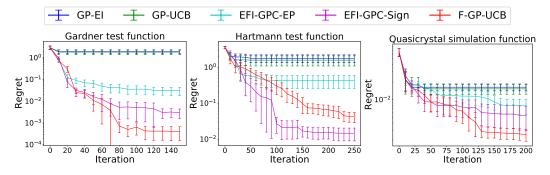
Figure 3: Experiment results of benchmark function of the constrained optimization problems (left and middle) and quasicrystal simulation function (right). The left and middle plots show the result of Gardner and Hartmann test functions, respectively. The error bars correspond to two standard errors.
