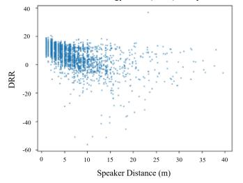
Figure 9: **DRR vs. Speaker distance.** We plot the Direct-to-Reverberant Energy Ratio (DRR) as a function of the distance between the source and receiver for SoundSpaces-Speech audio samples. As the distance between speaker and receiver increases, the listener receives more reverberant sound than direct sound from the speaker, leading to the observed decrease in DRR.
