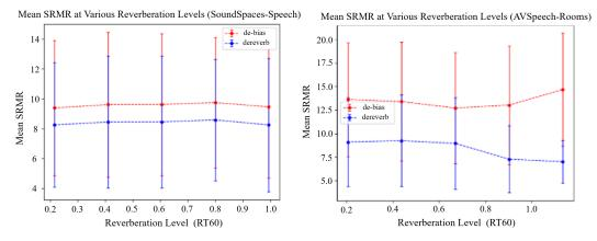
Figure 11: **De-biaser performance at various reverberation levels.** We stratify samples from both datasets by their RT60 and compute the mean SRMR scores of dereverberated and de-biased data within each bin. De-biased audio consistently produces higher SRMR scores than dereverberated audio across all reverberation levels and datasets.
