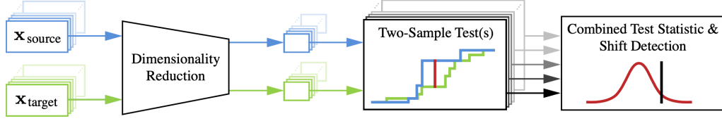
Figure 3: The procedure of detecting a dataset shift using dimensionality reduction and then a two-sample statistical test. The dimensionality reduction is applied to both the detection-training (source) and test (target) data, prior to being analyzed using statistical hypothesis testing. This figure is taken from [37].
