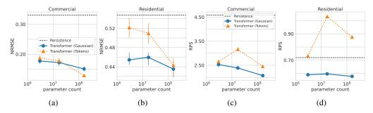
Figure 8: Model size vs. Buildings-900K-Test zero-shot STLF performance. Intervals are 95% stratified bootstrap CIs of the median. The trends in (a)-(c) suggest superior generalization to the test data is achievable by larger models, which might be unsurprising due to the *small* distribution shift between the simulated pretraining and simulated test data (relative to the *large* distribution shift between the simulated pretraining and real test data).
