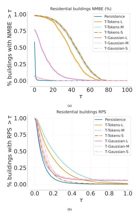
Figure 15: Real residential building zero-shot NMBE and RPS performance profiles with 95% bootstrap CIs. Curves closer to the bottom left are better.
