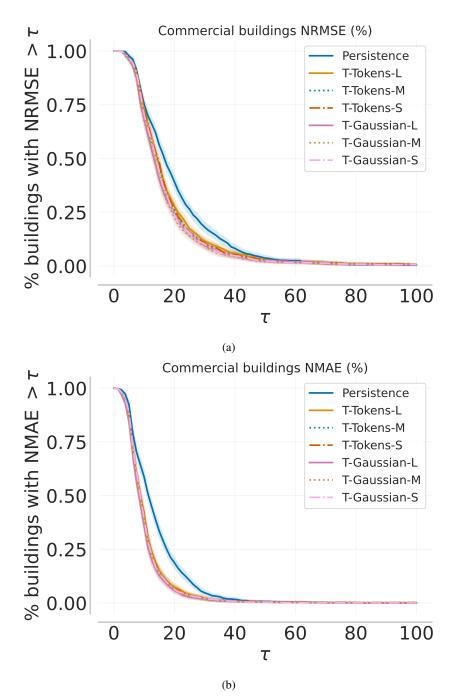
Figure 12: Real commercial building zero-shot NRMSE and NMAE performance profiles with 95% bootstrap CIs. Curves closer to the bottom left are better.
