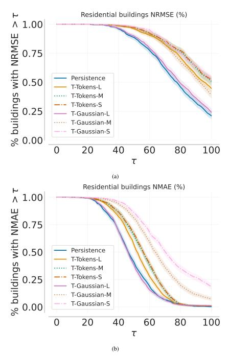
Figure 14: Real residential building zero-shot NRMSE and NMAE performance profiles with 95% bootstrap CIs. Curves closer to the bottom left are better.
