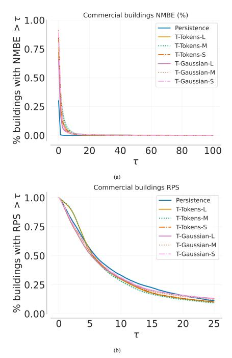
Figure 13: Real commercial building zero-shot NMBE and RPS performance profiles with 95% bootstrap CIs. Curves closer to the bottom left are better.
