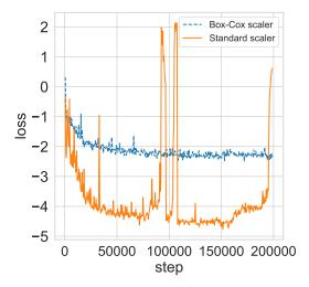
Figure 9: **Box-Cox scaling vs. standard scaling training stability**. Standard normalizing the load values did not prevent the Transformer (Gaussian) model from suffering from training instability. Box-Cox scaling was successful at achieving stable training.
