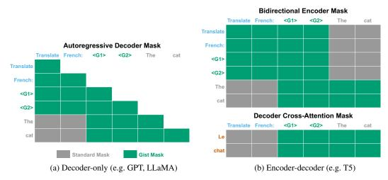
Figure 2: **Gist Masking**. Attention mask modifications for (a) decoder-only and (b) encoder-decoder Transformer LMs to encourage prompt compression into gist tokens  $\langle G1 \rangle \langle G2 \rangle$ . In these tables, cell (r, c) shows whether token r can attend to token c during self- or cross-attention.
