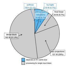
Figure A.4: **FLOPs for each operation involved in a single layer of self attention with a 2000-length KV cache**, according to the Chinchilla estimates for LLaMA-7B. At most 9.6% of FLOPs can be optimized away by reducing the size of the KV cache.
