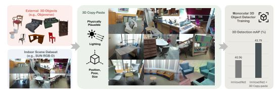
Figure 1: Overall pipeline of physically plausible object insertion for monocular 3D object detection: Our approach *copies* external 3D objects (e.g., from Objaverse [Deitke et al., 2022]) and *pastes* them into indoor scene datasets (e.g., SUN RGB-D [Song et al., 2015]) in a physically plausible manner. The augmented indoor scene dataset, enriched with inserted 3D objects, is then used to train monocular 3D object detection models, resulting in significant performance improvements.
