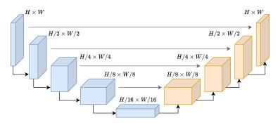
Figure 9: The architecture of U-Net contains four downsampling and upsampling operations.
