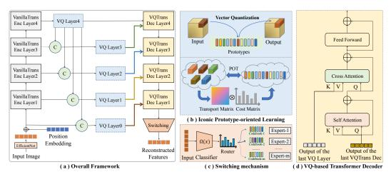
Figure 2: (a) The overall framework of our HVQ-Trans. (b) Each VQ-based Layer replaces continuous features with iconic prototypes, equipped with the POT module to promote better learning and scoring. (c) The codebook and expert network are switched for individual image. (d) The detailed structure of each VQ-based Transformer decoder, where the prototypes are integrated via cross-attention.
