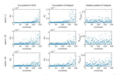
Figure 10: How the true gradient  $(\{|g_{i_k}|\}_{k=1}^d)$  and "adaptive gradient"  $(\{|g_{adapt,i_k}|\}_{k=1}^d)$  align with diagonal of Hessian  $(\{|H_{i_k,i_k}|\}_{k=1}^d)$ . Here coordinates are sorted such that  $|H_{i_1,i_1}| \leq |H_{i_2,i_2}| \leq \dots \leq |H_{i_d,i_d}|$  (suppose  $H \in \mathbb{R}^{d \times d}$ ). Experiments were conducted on the model described in Section A.1. This figure shows the results on the 12-th layer.
