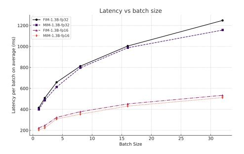
Figure 2: Inference latency with batch implementation in A100 GPU with fp32 and fp16 format.
