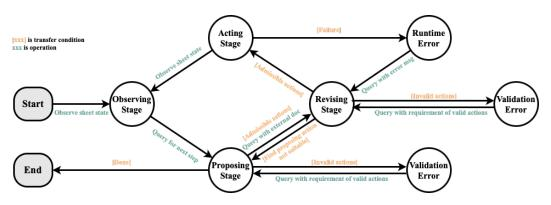
Figure E: The complete state machine for task planning. The transfer condition (orange texts with brackets) must be fulfilled before performing the corresponding operation (green texts) to transfer to a next state.
