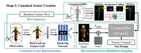
(a) **Canonical Avatar Creation.** We randomly sample a camera viewpoint to render both the 3D avatar and an SMPL model. The extracted SMPL 3D keypoints are projected to a 2D skeleton image with occlusion culling. The skeleton image is by construction 3D-consistent with the rendered avatar. We then utilize ControlNet [48] conditioned on the text prompt and the skeleton image instead of the original SD [34].
