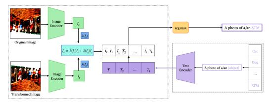
Figure 1: Implementation of  $\lambda$ -equitune on CLIP. Weighted average of image features corresponding to transformed inputs are computed, which is further used for computing text-image similarity scores.
