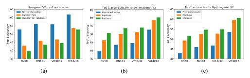
Figure 4: In (a) note that zero-shot performance of CLIP drops significantly when we add random rotations or flips to the input. This trend is seen across all image encoders, i.e. ResNet (RN50 and RN101) and ViT (ViT-B/32 and ViT-B/16). In (b) and (c) we show classification results on Imagenet-V2 with random 90° rotations and flips, respectively. We observe equizero outperform equitune and original CLIP for all image encoders.
