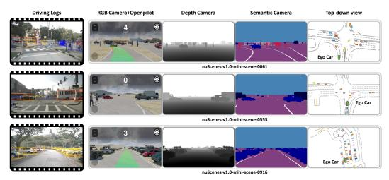
Figure 1: Snapshots of three scenarios extracted from *nuScenes* and their corresponding interactive environments with multiple views and sensors including RGB camera, depth camera, and semantic camera. The RGB sensor can be used for end-to-end driving systems like Openpilot [10].
