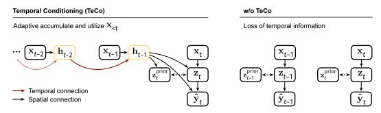
Figure 5: Graphical illustration of the temporal conditioning operation (TeCo). After completely excluding the temporal dimension from the model parameter space, we introduced the temporal conditioning operation to handle the temporal information. In particular, this operation enables *memory-dependent processing* as in biological coding circuits.
