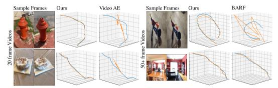
Figure 3: **Qualitative Pose Estimation Comparison**. On short sequences, we compare our pose estimation to Video Autoencoder [53], and on long sequences, we compare our method's sliding-window estimations against the per-scene optimization BARF [38]. The trajectory for the bicycle sequence was obtained using a model trained on hydrant sequences: despite never having seen a bicycle before, our model predicts accurate poses.
