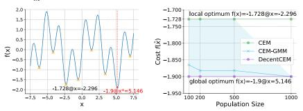
Figure 3: Left: The objective function in a 1D optimization task. Right: Comparison of the proposed DecentCEM method to CEM and CEM-GMM, wherein the line and the shaded region denote the mean and the min/max cost from 10 independent runs.  $\hat{x}$ : solution of each method.
