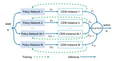
Figure 5: The architecture of DecentCEM planning with M CEM instances.  $\psi_i = \phi_i$  for planning in action space and  $\psi_i = \theta_i$  for planning in policy network parameter space with the instance index  $i \in \{1, \dots, M\}$ .
