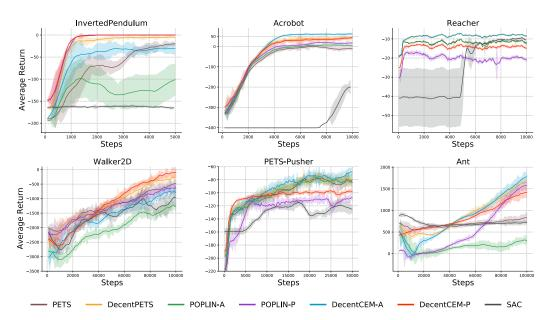
Figure 6: Learning curves of the proposed *DecentCEM* methods and the baselines on continuous control environments. The line and the shaded region shows the mean and standard error of evaluation results from 5 training runs with different random seeds.
