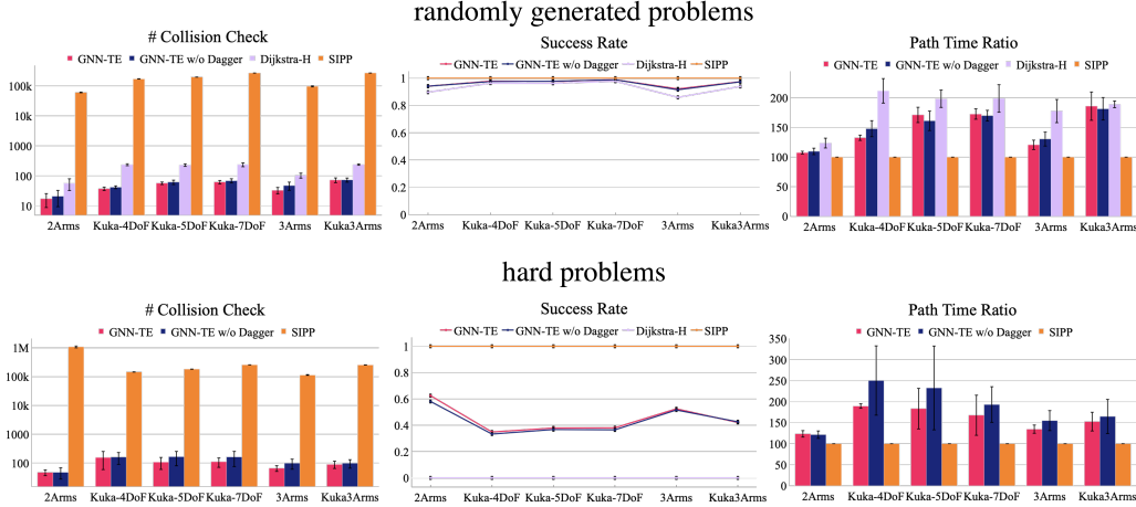
Figure 4: Overall Performance of baselines on collision checking, success rate, and path time ratio. Our approach significantly reduces collision checking more than 1000x compared to the complete algorithm SIPP, improves the overall planning efficiency, and achieves high success rates.
