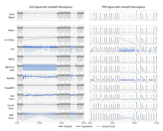
Figure 1: Visualization of imputation results on ECG and PPG signals. The large gaps found in real-world missingness patterns create substantial challenges for all methods. BRITS and DeepMVI produce nearly constant outputs. GAN-based approaches (BRITS w/ GAIL and NAOMI) hallucinate incorrect structures in incorrect locations. Our BDC Transformer also struggles in the middle of long gaps, but has the strongest performance overall, most closely reconstructing the ground-truth.
