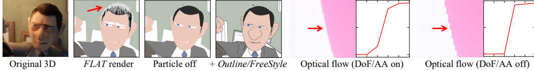
Figure 3: Illustrations on some design choices. In our data, 2D cartoon frames are rendered under the “ FLAT ” lighting of Workbench engine in Blender. Particle effects that simulate real small objects are turned off for a more similar looking of real cartoons. Depth of field (DoF) and Anti-Aliasing (AA) are turned off for sharp optical flow boundary.
