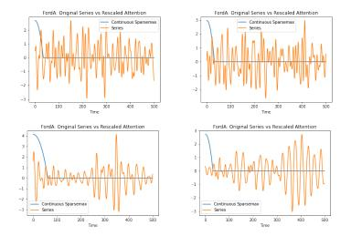
Figure 5: Original time series vs rescaled attention densities for four randomly selected examples from the FordA dataset using continuous sparsemax. The densities are rescaled so that they have the same max as the signal. The densities are again simple and do not attend to fine portions of the signal, although have more focus than in the continuous softmax case.
