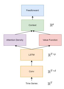
Figure 11: Architecture used for the MIT BIH and FordA experiments. The input is a univariate time series. The conv block has two conv layers, with the goal of converting a univariate time series into a multivariate one. The hidden units of the LSTM are then used to compute the attention density parameters and the value function. The feedforward network has three layers, where the first two have ReLU activation functions.
