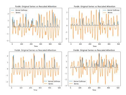
Figure 7: Original time series vs rescaled attention densities for four randomly selected examples from the FordA dataset using kernel softmax. The densities are rescaled so that they have the same max as the signal. The densities seem to focus often on the zero crossings where the signal moves from a peak to a trough.
