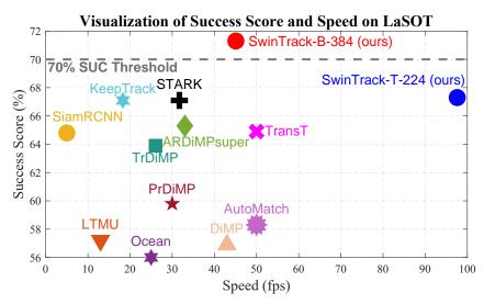
Figure 1: Comparison on LaSOT [9]. Our tracker (SwinTrack-B-384) sets a new record with 0.713 SUC score and still runs efficiently at around 45 *fps*. A lighter version (SwinTrack-T-224) achieves 0.672 SUC score and runs at around 96 *fps*, which is on par with existing SOTAs in accuracy but much faster.
