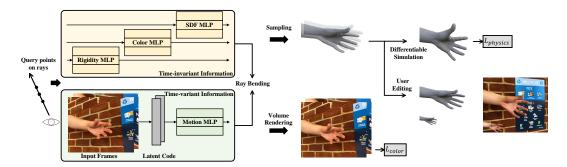
Figure 1: **Overall workflow**. *NeuPhysics* takes a monocular video as supervision. The time-invariant fields are defined on a reference frame, while time-dependent motion is applied to each point sampled in space. We then compute color loss from the volume rendered images. A differentiable simulator is embedded after optimizing the neural fields, to learn dynamics parameters and allow scene editing. A detailed computational graph can be found in Figure 3.
