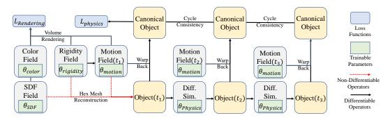
Figure 3: **Computational Graph During Training.** We show how data transfers among modules in a basic 3-step dynamical systems. All operators are differentiable, except the hex mesh reconstruction for the first frame. In our designed cycle consistency mechanism, the rigidity and motion networks serve as the bridge between the rendering and physics module.
