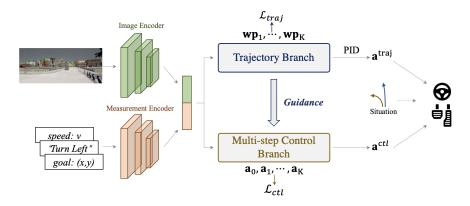
Figure 2: Overview of Trajectory-guided Control Prediction (TCP). The encoded features are shared by the trajectory and multi-step control branch. The trajectory branch provides per-step guidance for multi-step control prediction. Outputs from two branches are combined according to our situation based fusion scheme to generate the ultimate control actions.
