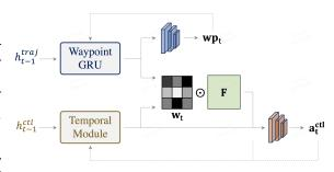
Figure 3: Detailed trajectory guiding process. For predictions at time step t, the hidden states from the waypoint GRU and the temporal module are combined to learn an attention weight map to re-aggregate the 2D image feature map for control prediction.
