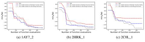
Figure 5: The performance of PSO, our meta-optimizer trained on Rastrigin function family and that trained on real energy functions for three different levels of docking cases: (a) rigid (easy), (b) medium, and (c) flexible (difficult).
