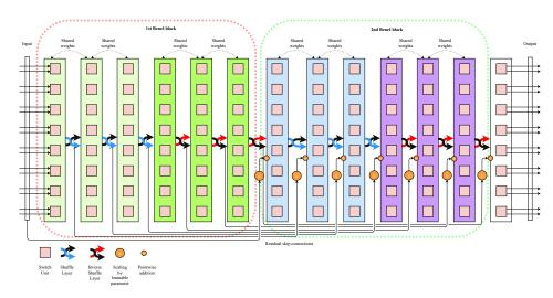
Figure 3: Neural Shuffle-Exchange network with 2 Beneš blocks.
