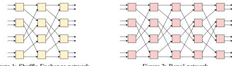
Figure 1: Shuffle-Exchange network.
