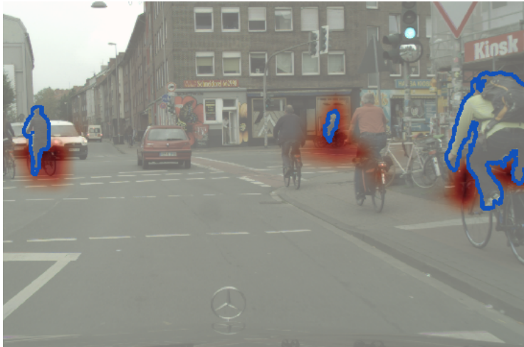
Figure S12: Influence of the size of the request mask R on context explanations provided by grid saliency. Independent of the request mask R size, for all riders salient context always falls on bikes. Note that the context grid saliency explanations were calculated for each request region separately and are only combined together for the visualization.
