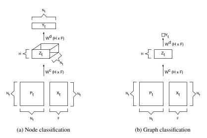
Figure 1: DCNN model definition for node and graph classification tasks.
