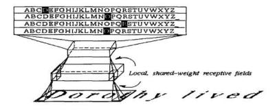
Figure 3: Net architecture for parallel character sequence classification, n=4 chars.
