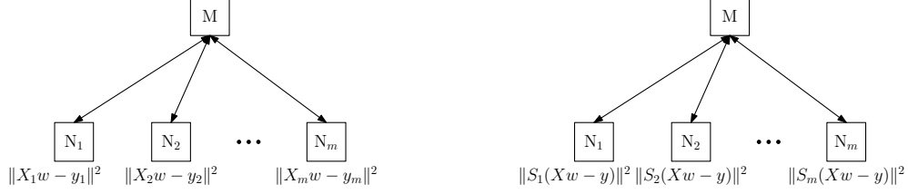
Figure 1: Left: Uncoded distributed optimization with partitioning, where X and y are partitioned as X = [X_1^\top X_2^\top \dots X_m^\top]^\top and y = [y_1^\top y_2^\top \dots y_m^\top]^\top . Right: Encoded distributed optimization, where node i stores (S_i X, S_i y) , instead of (X_i, y_i) . The uncoded case corresponds to S = I .
