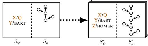
Figure 1: A module is mapping an upstream proof state (left) to a list of new proof states (right), thereby extending the substitution set  $S_\psi$  and adding nodes to the computation graph of the neural network  $S_\rho$  representing the proof success.
