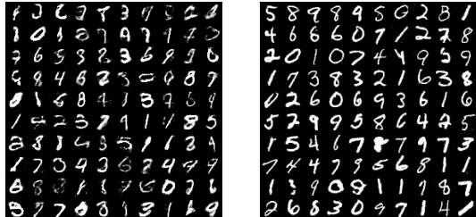
Figure 3: (Left) samples generated by model during semi-supervised training. Samples can be clearly distinguished from images coming from MNIST dataset. (Right) Samples generated with minibatch discrimination. Samples are completely indistinguishable from dataset images.
