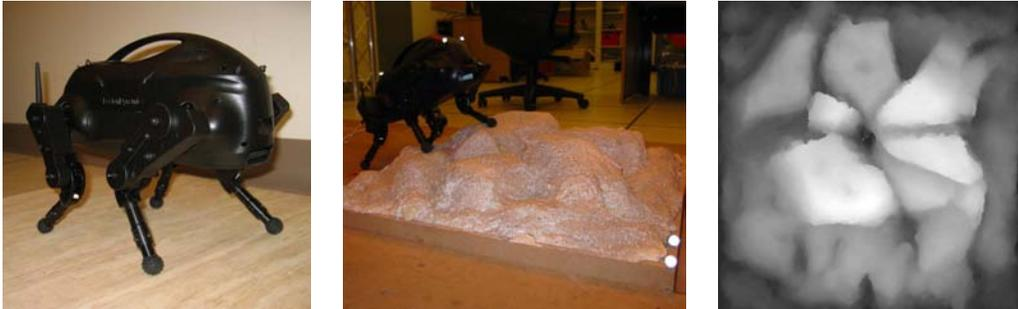
Figure 1: (a) LittleDog robot, designed and built by Boston Dynamics, Inc. (b) Typical terrain. (c) Height map of the depicted terrain. (Black = 0cm altitude, white = 12cm altitude.)
